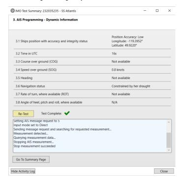
The **Test** button will start interrogating the selected AIS Transceiver for the Section 3 AIS message.
