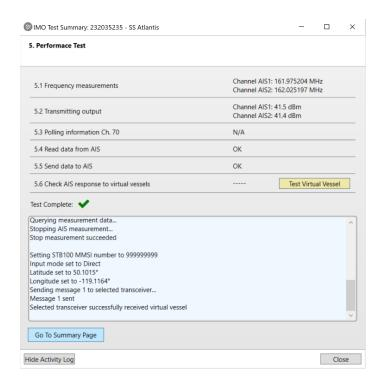
The **Test Virtual Vessel** button will send a position report message to the selected transceiver to emulate a ship in the area.
