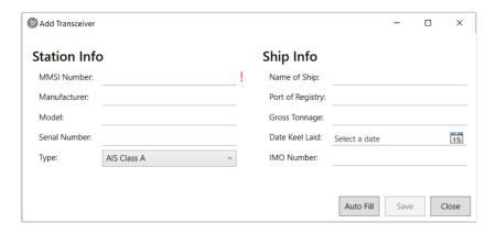
Press *Auto Fill*. The receiver will wait for the Transceiver signal transmission and extract the necessary details. Alternatively, the user manually completes the information, then clicks *Close*.
