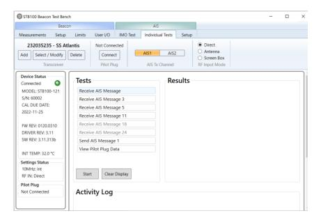
The main **Individual Test** screen allows users to run individual tests associated with AIS transceivers. This screen has 3 sections: Tests; Results; and Activity Log.
