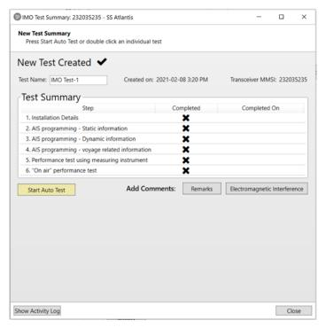
The **IMO Test Summary** window allows users to change the **Test Name**, start an *Auto Test*, view the **Activity Log** window, add **Test Remarks**, add **Electromagnetic Interference Comments**, view completion of individual test steps, and navigate to each section of the IMO Test Report.
