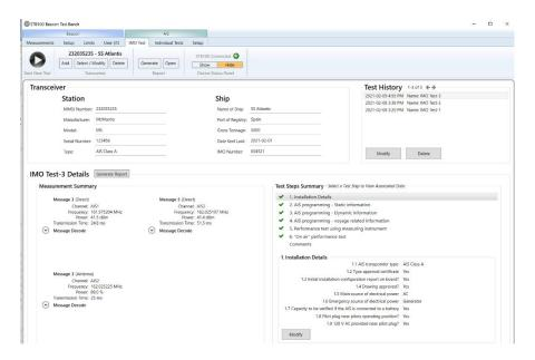
The main **IMO Test Screen** displays information based on the selected transceiver; test history associated with the selected transceiver; and a details section that includes measurement and IMO test related data for a selected test.
