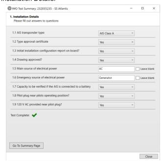
Section 1.1 auto selects the transceiver type based on which AIS transceiver class was specified when creating the associated transceiver.
