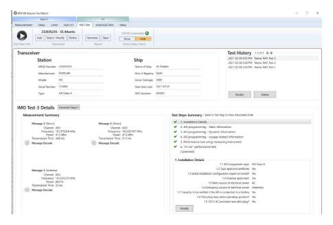
In the **Details - Measurement Summary** section, the user can review the RF measurement data and the decoded AIS data from each of the received messages.
