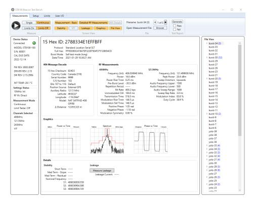
**Measurement – Basic** includes the Beacon Hex ID and all decode details, along with frequency and power of each selected channel.
