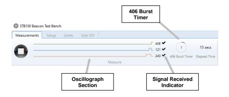
The 121, 243, and AIS signals must be received before a 406 burst. The measurement is deemed to be completed once the 406 burst is received.
