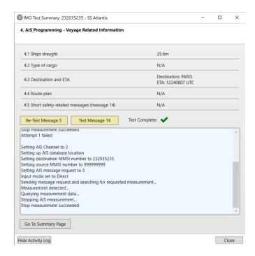
Section 4.5 requires a user to actively transmit a safety-related message (SRM) from the selected AIS Transceiver. To complete this section, click the **Test Message 14** button and transmit AIS message 14 from the selected transceiver. Please refer to the Transceiver's instruction manual for information on sending the SRM Message 14. Once Message 14 has been received, section 4.5 will update to 'OK'.
