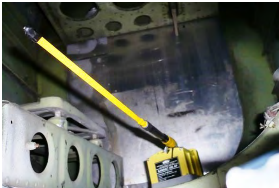
TEST 03 Horizontal antenna within tail boom
