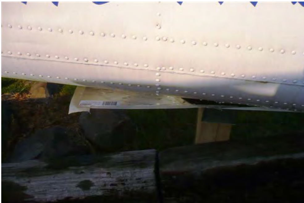
Duct tape came undone sometime during 24 hour test of Test 03 (as it is on the underside of antenna unlikely to influence test)
