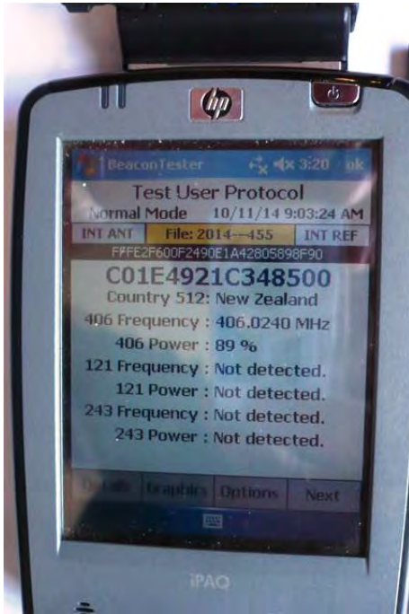
Test 03 2014-455 = 89% Power Test taken underneath tail boom
