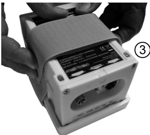
Figure 15: Installing the transmitter on the bracket
