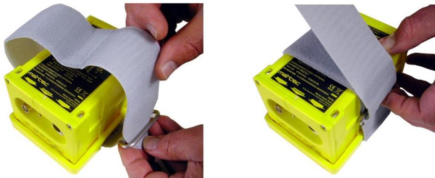
4. Ensure the buckle is correctly positioned (indifferently on right or left side of ELT) regarding the horizontal center line of ELT and firmly adjust and tighten the retaining strap.
