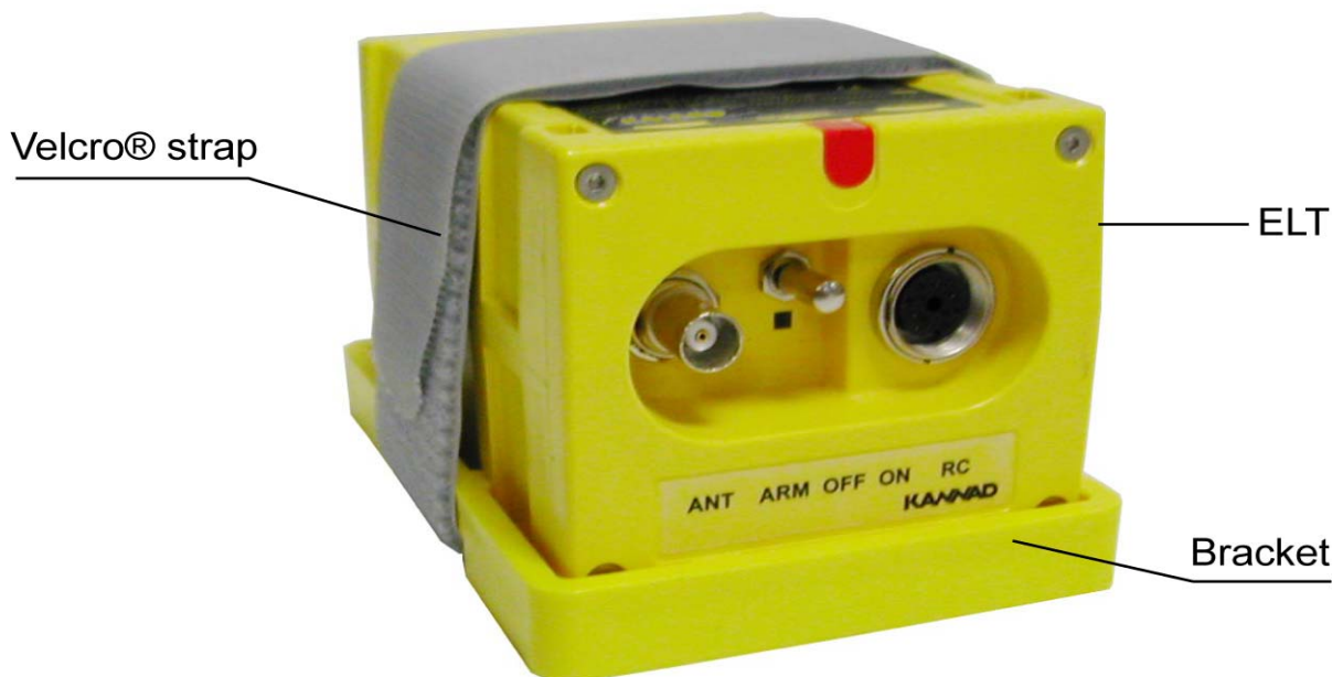
Figure 4: ELT Transmitter with Mounting Bracket
